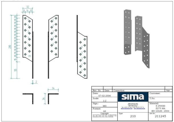
Additionally the bracket can be made from 1,5 mm pre-galvanized steel grades S350GD to Grade S500GD + min. Z275 according to EN 10346 named Purlin Anchor 210PL
