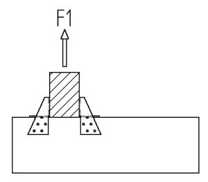
It is assumed that the beam is prevented from rotating. The brackets are intended for use for connections subject to static or quasi static loading.
