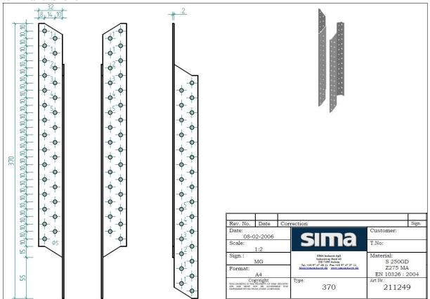
Additionally the bracket can be made from 1,5 mm pre-galvanized steel grades S350GD to Grade S500GD + min. Z275 according to EN 10346 named Purlin Anchor 370PL
