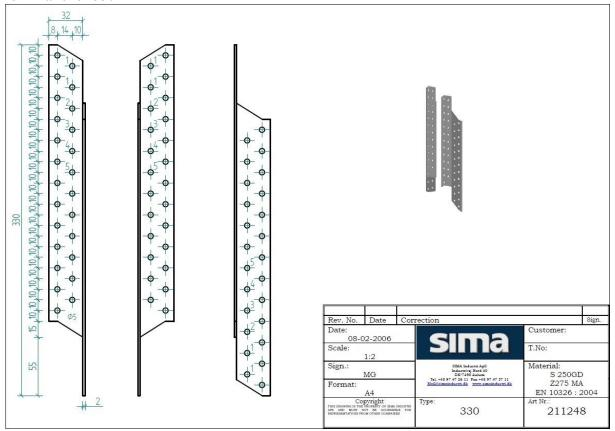
Additionally the bracket can be made from 1,5 mm pre-galvanized steel grades S350GD to Grade S500GD +  $\min$ . Z275 according to EN 10346 named Purlin Anchor 330PL
