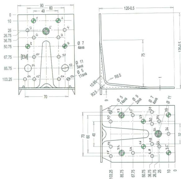
Figure B. 82 Dimensions of angle bracket
