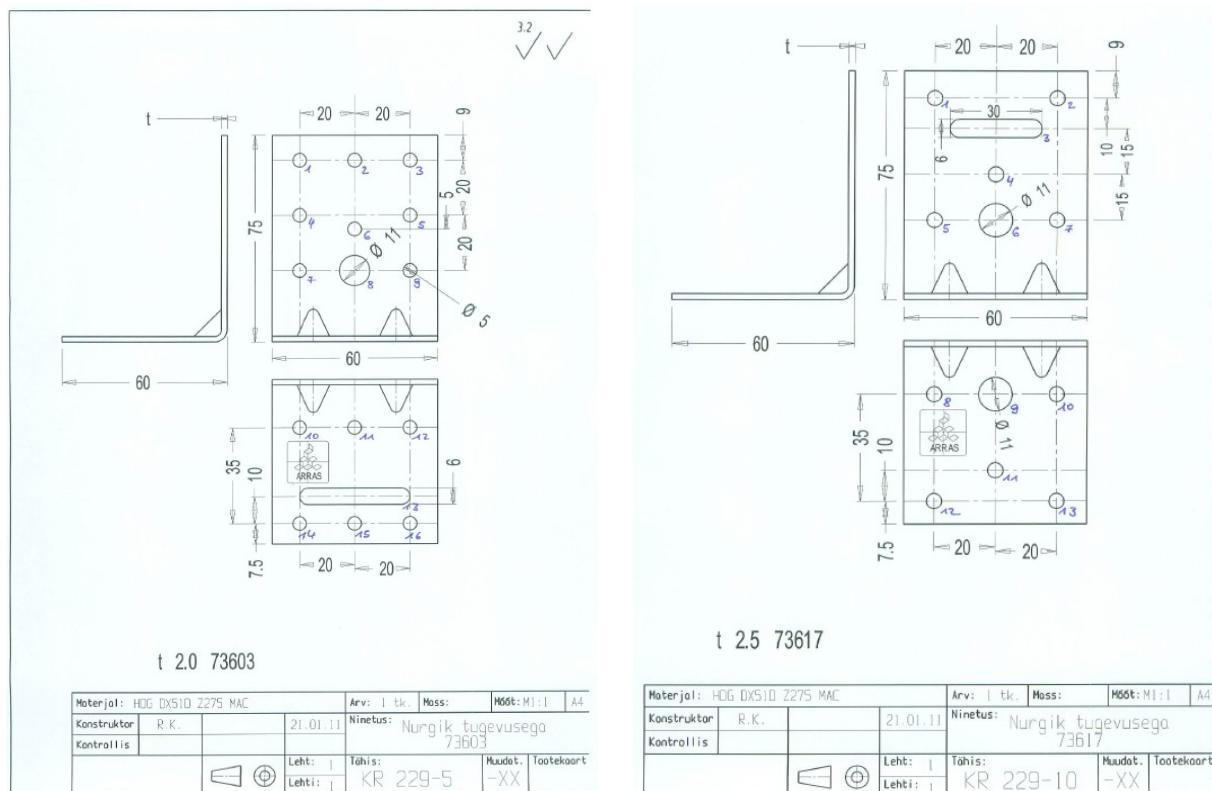
Figure B. 35 Dimensions of angle bracket
