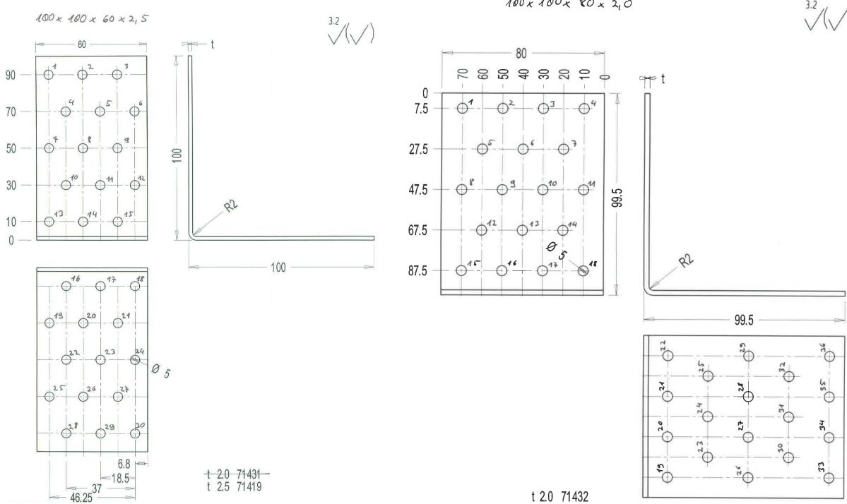
Figure B. 68 Dimensions of angle bracket
