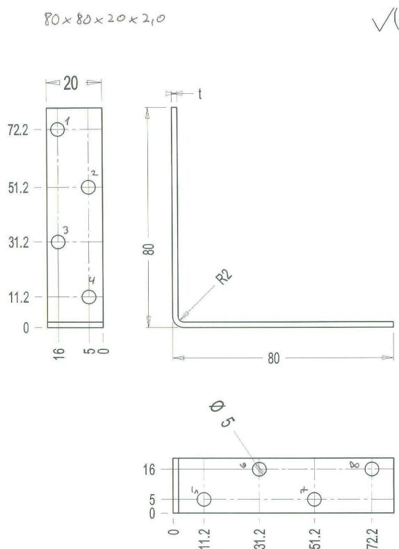
Figure B. 37 Dimensions of angle bracket
