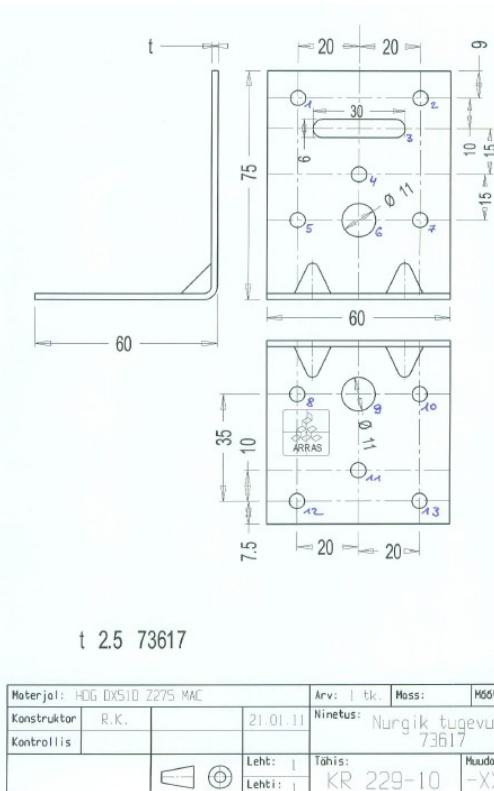
Figure B. 33 Dimensions of angle bracket
