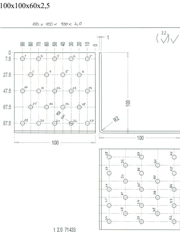
Figure B. 70 Dimensions of angle bracket
