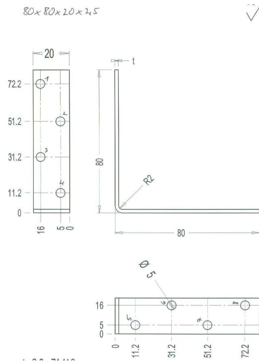
Figure B. 38 Dimensions of angle bracket
