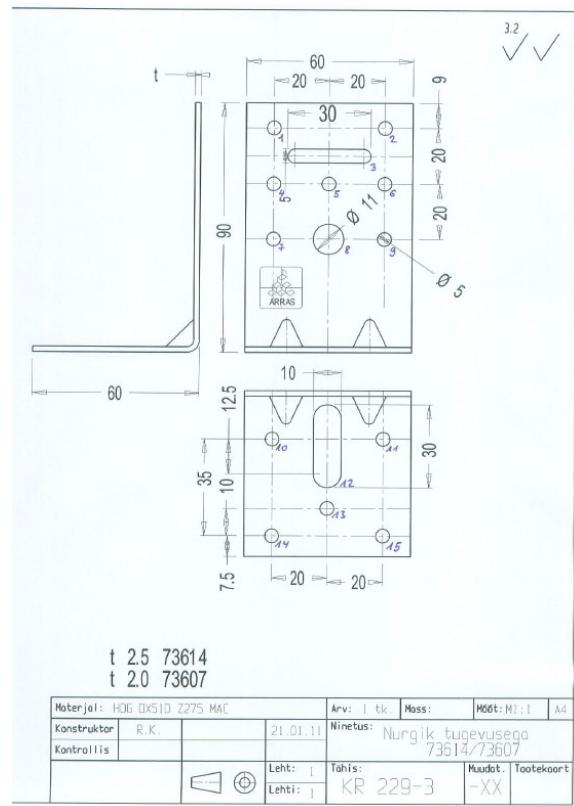
Figure B. 53 Dimensions of angle bracket
