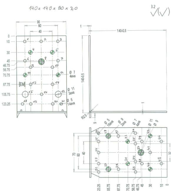
Figure B. 85 Dimensions of angle bracket
