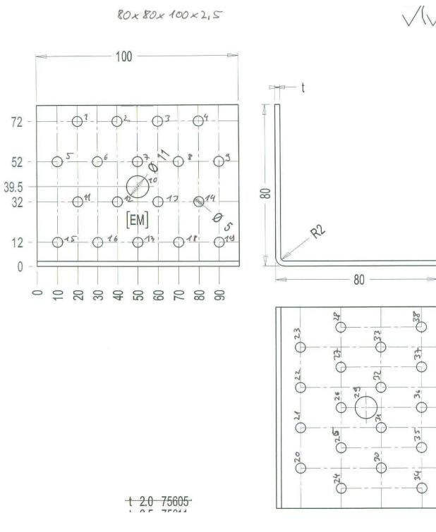
Figure B. 48 Dimensions of angle bracket
