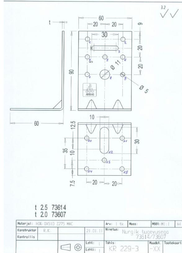
Figure B. 51 Dimensions of angle bracket
