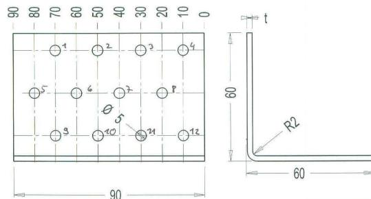
Figure B. 27 Dimensions of angle bracket
