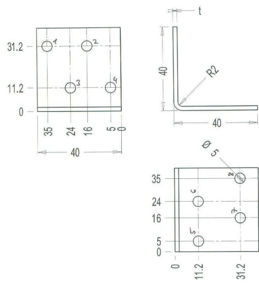
Figure B. 1 Dimensions of angle bracket
