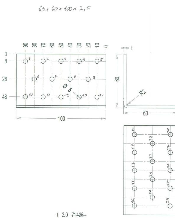
Figure B. 30 Dimensions of angle bracket
