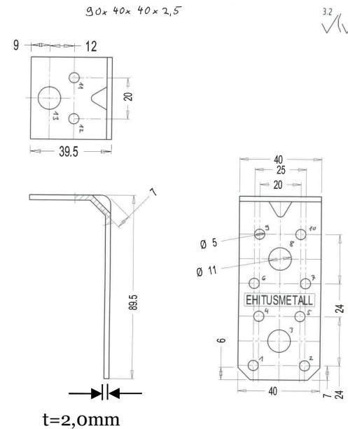
Figure B. 49 Dimensions of angle bracket
