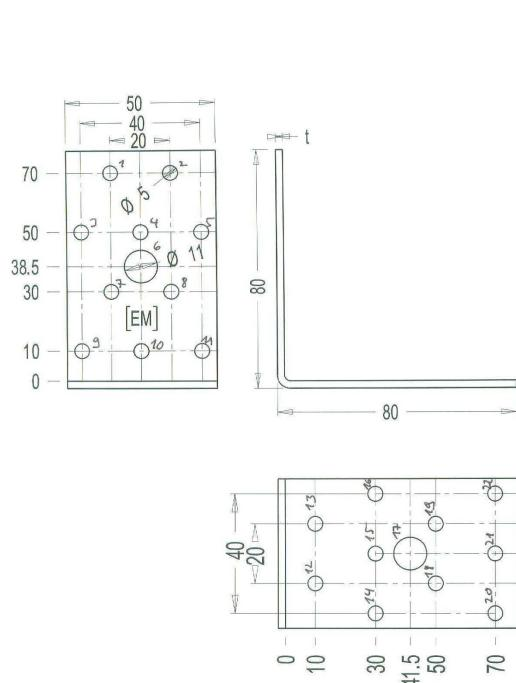
Figure B. 42 Dimensions of angle bracket
