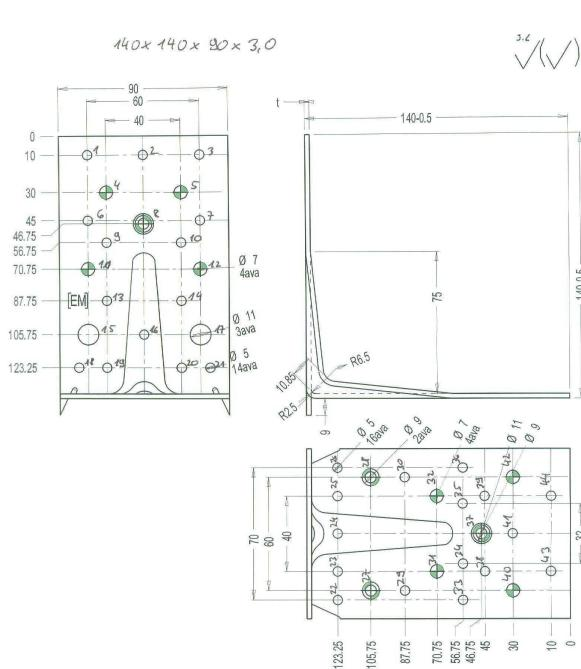
Figure B. 87 Dimensions of angle bracket
