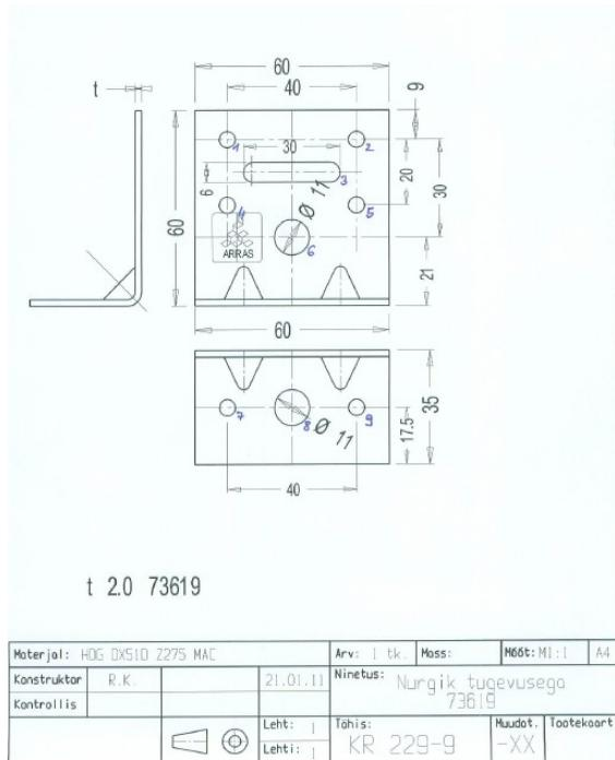
Figure B. 12 Dimensions of angle bracket
