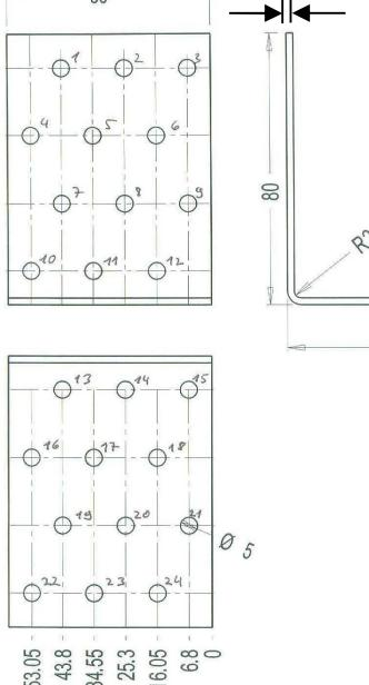
Figure B. 43 Dimensions of angle bracket
