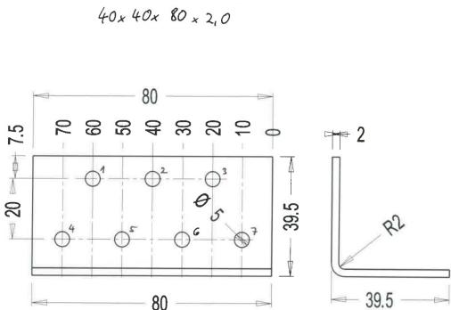
Figure B. 7 Dimensions of angle bracket
