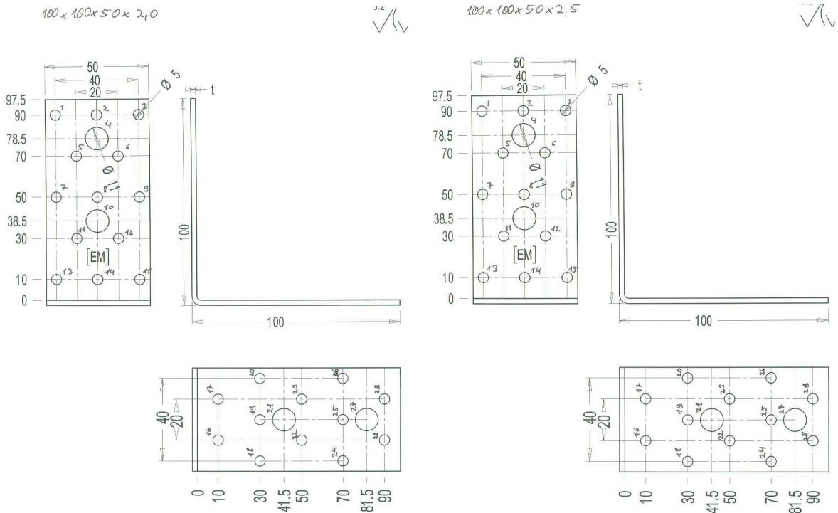
Figure B.64 Dimensions of angle bracket
