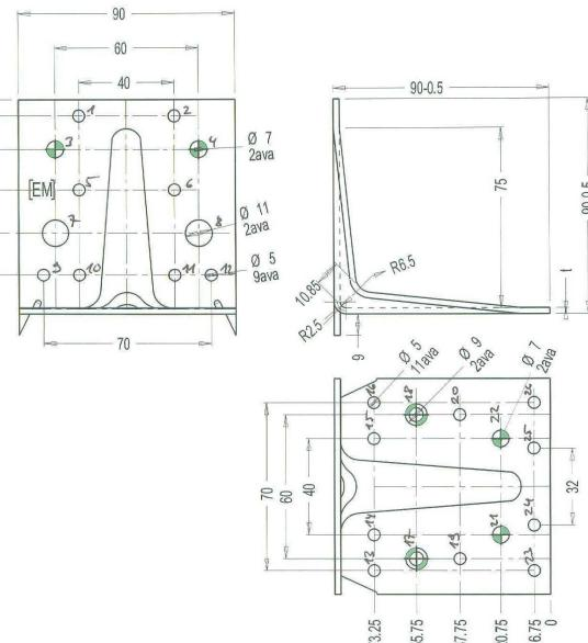
Figure B. 61 Dimensions of angle bracket
