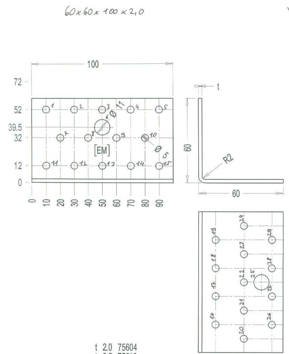
Figure B. 29 Dimensions of angle bracket
