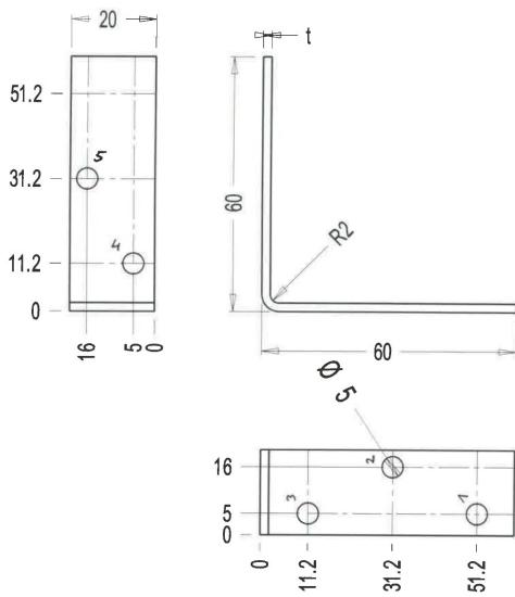
Figure B. 15 Dimensions of angle bracket
