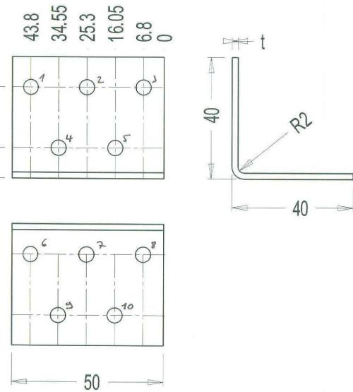
Figure B. 4 Dimensions of angle bracket
