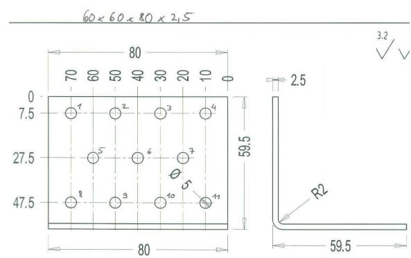
Figure B. 24 Dimensions of angle bracket
