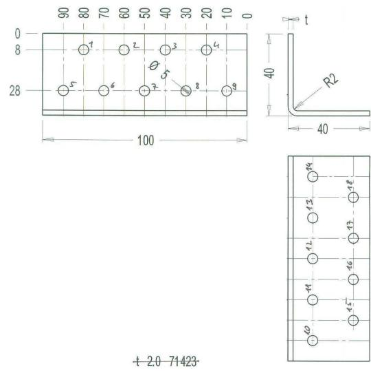
Figure B. 10 Dimensions of angle bracket
