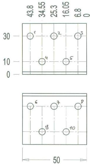
Figure B. 3 Dimensions of angle bracket
