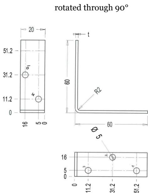
Figure B. 16 Dimensions of angle bracket
