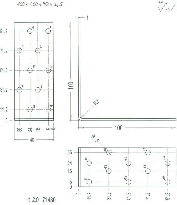
Figure B. 63 Dimensions of angle bracket
