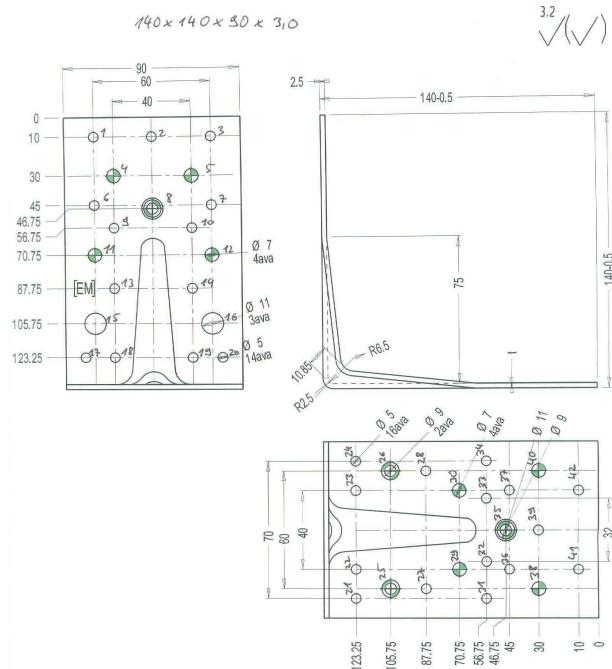
Figure B. 86 Dimensions of angle bracket
