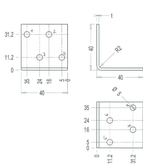
Figure B. 2 Dimensions of angle bracket
