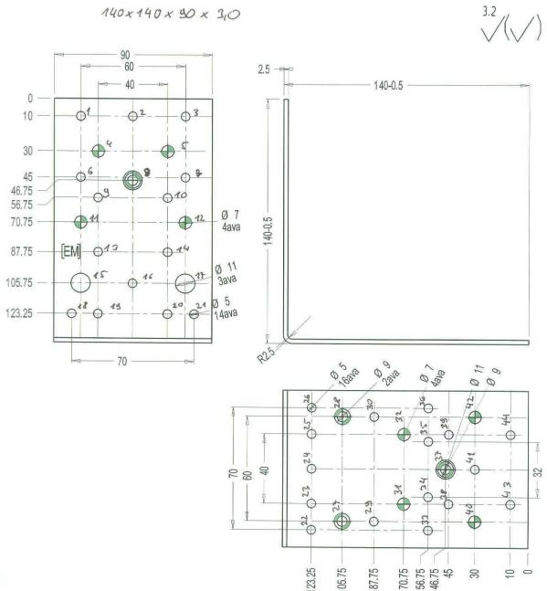
Figure B. 84 Dimensions of angle bracket
