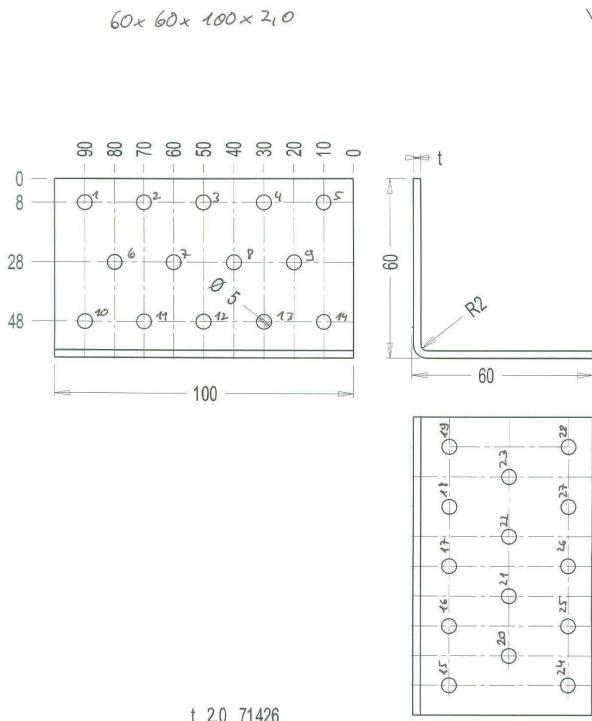
Figure B. 28 Dimensions of angle bracket
