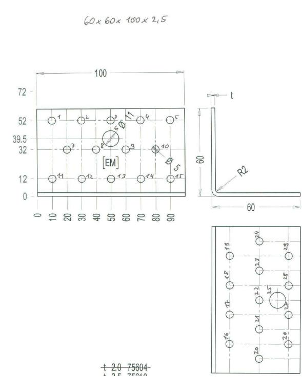
Figure B. 31 Dimensions of angle bracket
