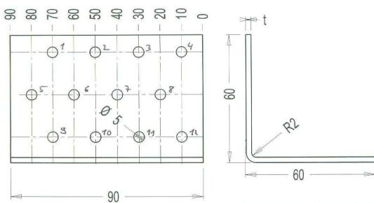
Figure B. 26 Dimensions of angle bracket
