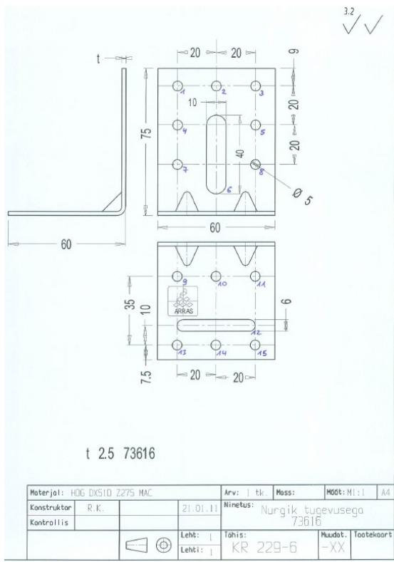
Figure B. 36 Dimensions of angle bracket
