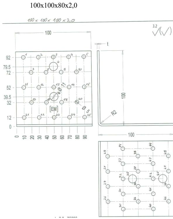
Figure B. 71 Dimensions of angle bracket
