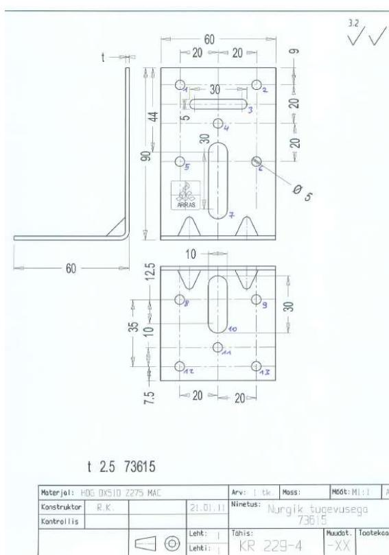
Figure B. 54 Dimensions of angle bracket
