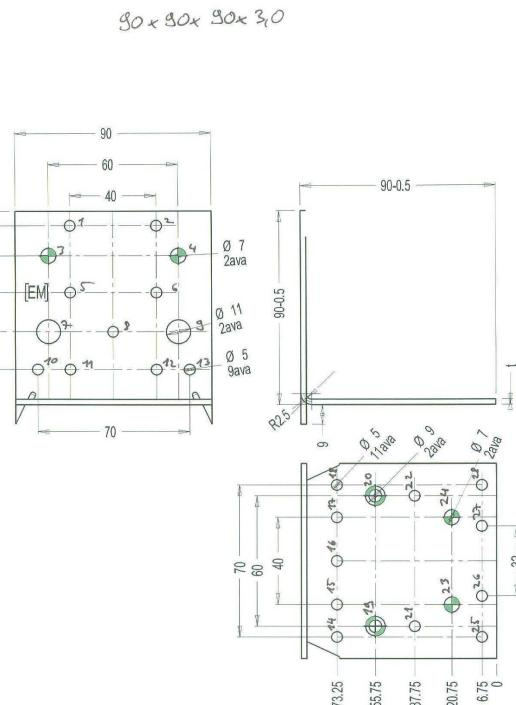
Figure B. 59 Dimensions of angle bracket
