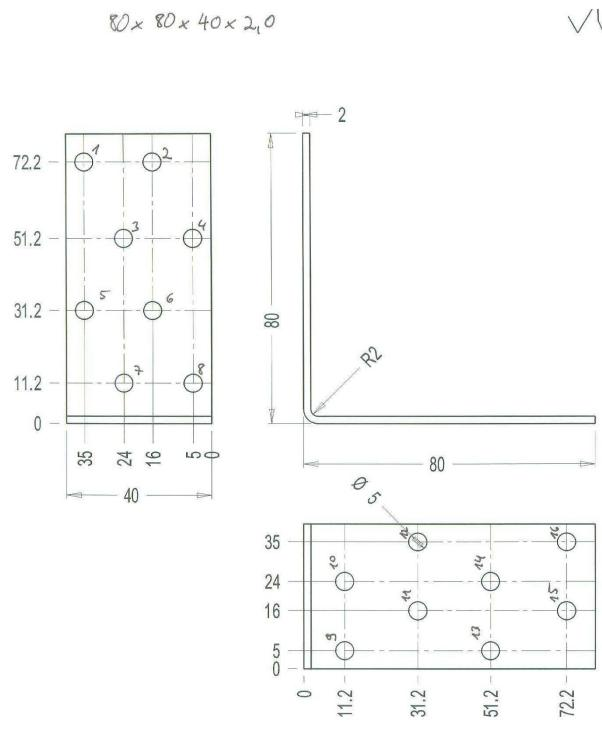
Figure B. 39 Dimensions of angle bracket
