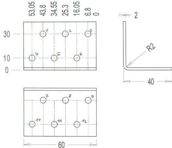
Figure B. 5 Dimensions of angle bracket
